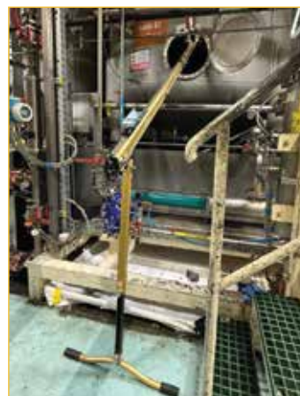
360° adjustable head with anchor/tie-off points.
