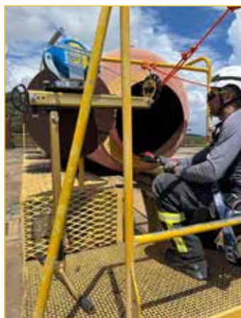
Adjustable mast and stabilizer mounting bracket.
