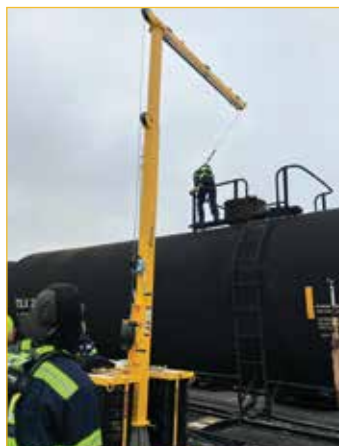
Portable with its counterweight system.
